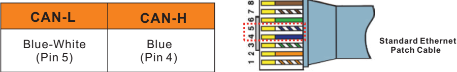
Figure 5.31 Battery Communication Wire Color Chart
