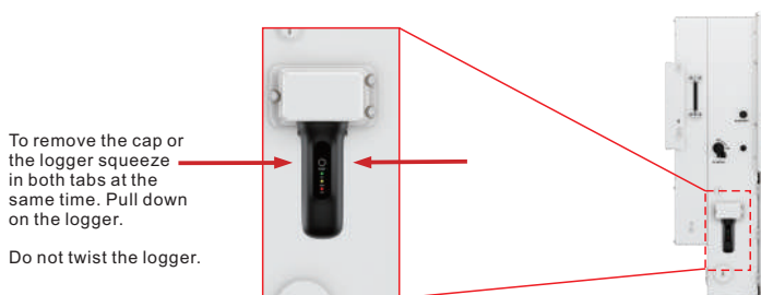
Figure 6.1 Solis data logger installation location
