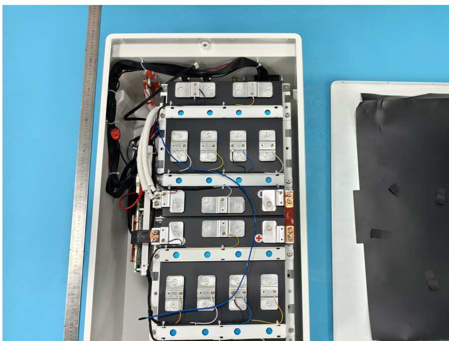
Figure 3 Battery interior view of LF51314A
