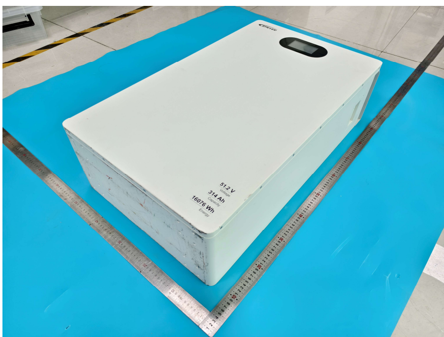
Figure 1 Front view of battery module of LF51314A
